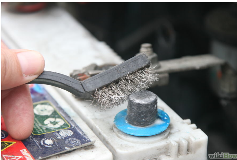
Figure 2 - Cleaning the Connection
